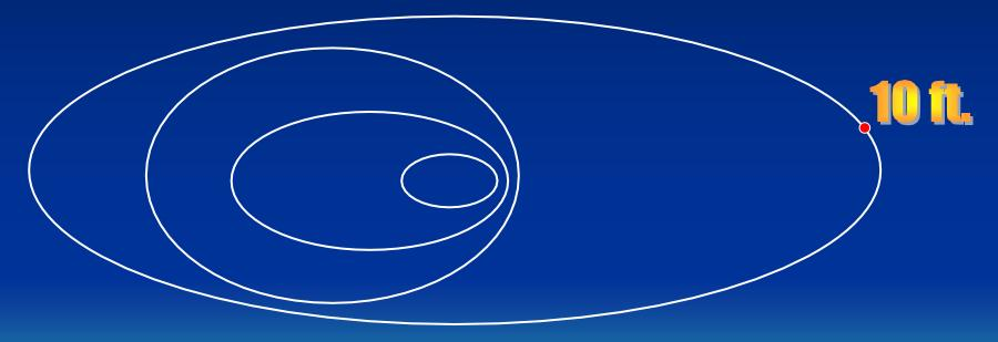
The increment in height from one contour line to the next called the
