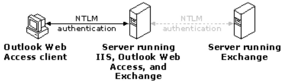
**Figure 6:** Accessing resources using NTLM authentication
